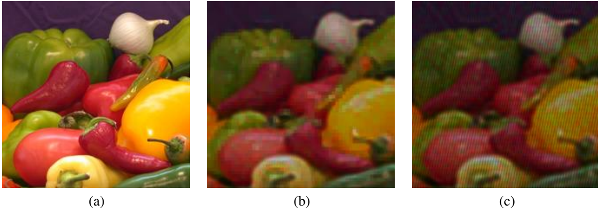
Figure 10. Spatio-spectral reconstruction results, color projections. (a) Color projection of true spatio-spectral data cube. (b) Color projection of estimated spatio-spectral data cube, computed using reconstruction method described above with multiscale spatio-spectral regularization. (c) Color projection of estimated spatio-spectral data cube, computed using reconstruction method described above with no regularization.
