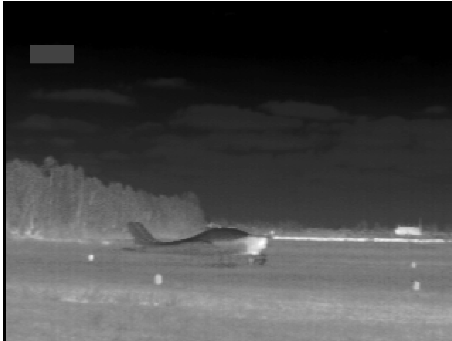
Figure 12 – A TECNAM P-2002 during take-off in an image taken by the IR camera
