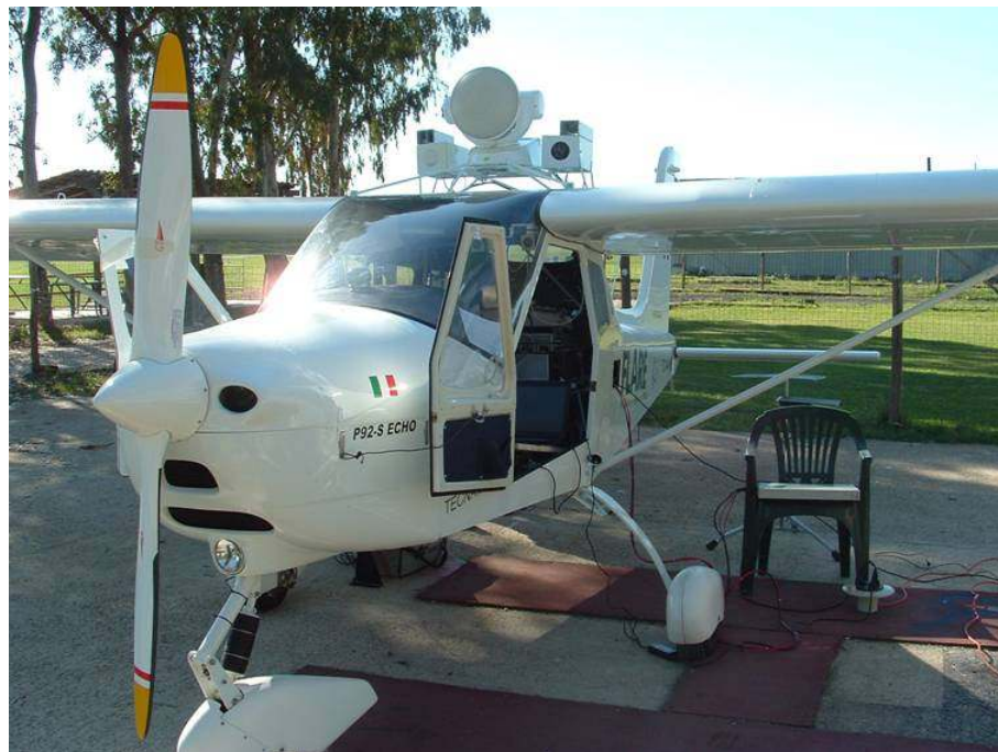
Figure 9 - Obstacle detection sensors mounted on-board FLARE
