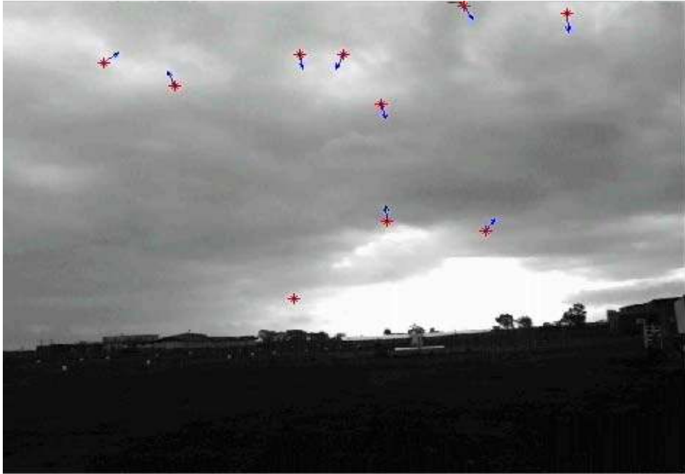
Figure 13 – Multiple false alarms in critical illumination conditions
