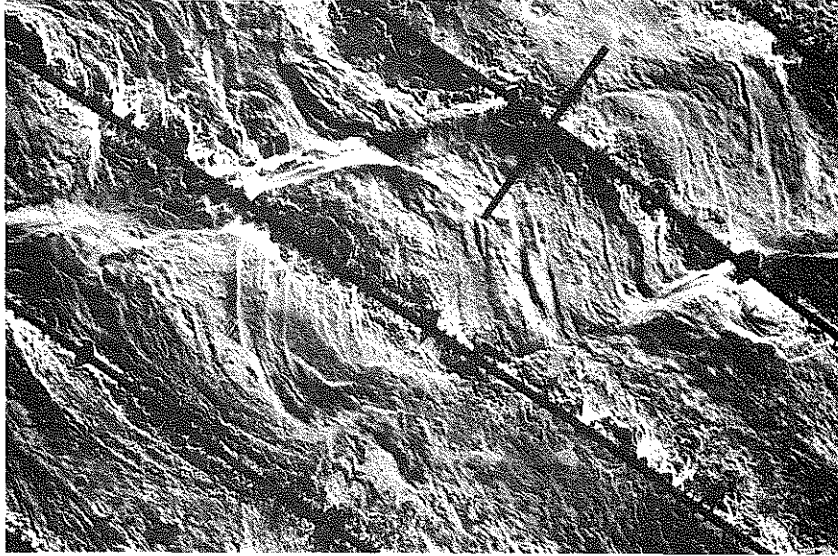
Figure 5.14: Sea MARC II: sidescan intensity (small-scale).
