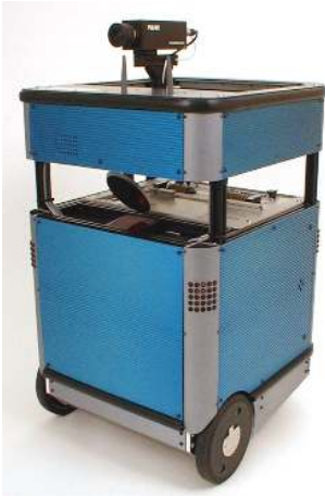
Figure 3: Pygmalion , the robot which was used in the experiments. It is a VME based system carrying currently a PowerPC card at 300 MHz. Besides wheel encoders and bumpers, the sensory system includes a 360° laser range finder and a gray-level CCD camera discussed in the second chapter. During the experiments it ran in a fully autonomous mode.
