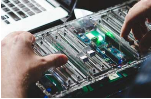
Fig. 14: The 8 x 1-Dof FireFader system built by Berdahl for his piece Transmogrified Strings .
