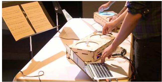
Fig. 16: Two Haptic Capstans (1-Dof rotary haptic devices) used in Andrew Pfalz’s Of Grating Impermanence .
