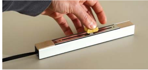
Fig. 8: The FIREFADER, a 1 DoF open-hardware haptic device based on a motorised slider and arduino micro-processor. Edition specifically built for Ableton's Loop festival by Alexandros Kontogeorgakopoulos and Odysseas Kleissouras.
