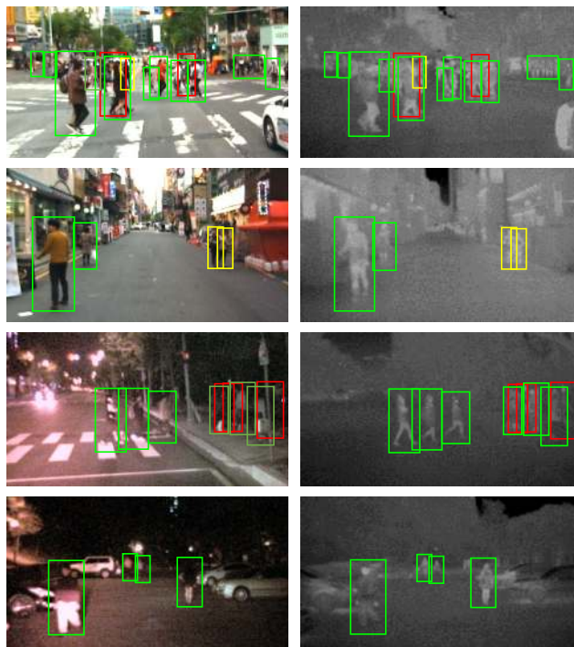
Figure 1. Examples of our multispectral pedestrian dataset . It has aligned pair of color (left column) and thermal (right column) images captured from day/night traffic scenes. The dense annotations provided with the dataset such as green, yellow, and red boxes indicate no-occlusion, partial occlusion, and heavy occlusion respectively. Images are cropped for better visualization.
