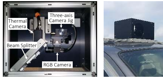
Figure 2. Our hardware configuration for capturing multispectral images. (Left) Top view. (Right) Mounted on the rooftop of a car.
