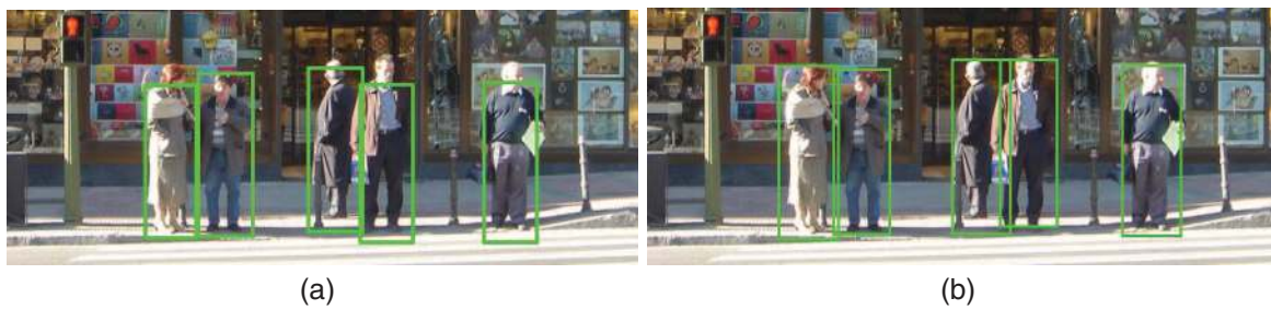
Fig. 10: Detection with SW (a) and with MS-PW (b) on an example image taken from INRIA test dataset. MS-PW shows a remarkably higher localization of detections. Both runs generated 1 false positive in the image, that has been removed for clarity of depiction.
