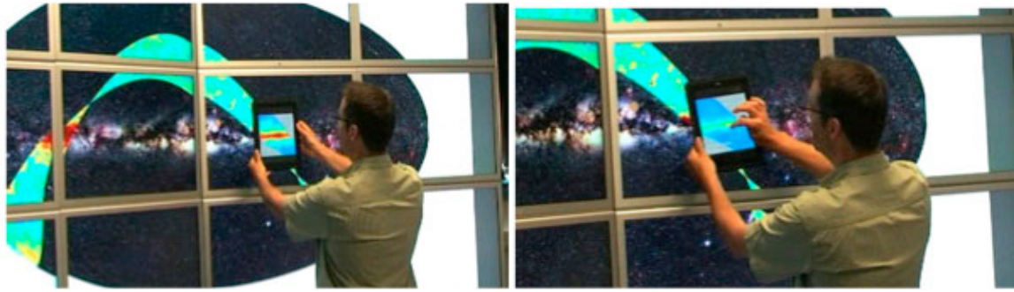
Figure 1: Using the Wizard of Oz technique to prototype how a tablet can serve as a mobile, physical filter atop a wall-sized image.
