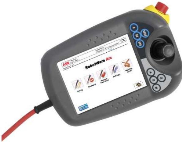
Figure 2.8: An example of a teach pendant: The ABB IRC5 FlexPendant.
