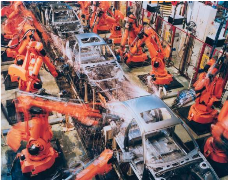
Figure 2.4: A spot-welding line using ABB IRB6400 robots.
