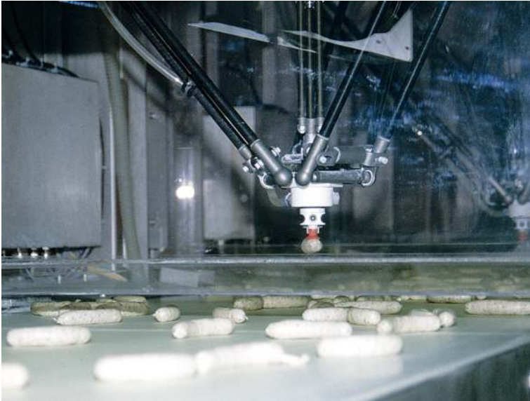
Figure 2.3: Picking sausages with the ABB IRB340 FlexPicker.
