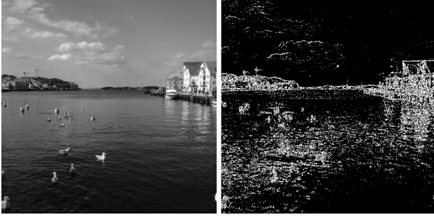
Fig. 1. Test image (left) and the embedding changes displayed in white when embedding relative payload 0.4 bpp (right).
