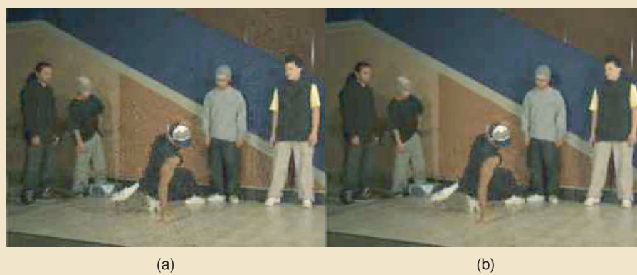
[FIG10] Decoded pictures of the multiview video Breakdancers . The subband coding scheme uses (a) the motion- and disparity-compensated lifted 5/3 wavelet or (b) the bidirectionally motion- and disparity-compensated orthogonal transform. In both cases, the same 8 \times 8 block motion/disparity field is used. View-temporal subbands are encoded with JPEG 2000.
