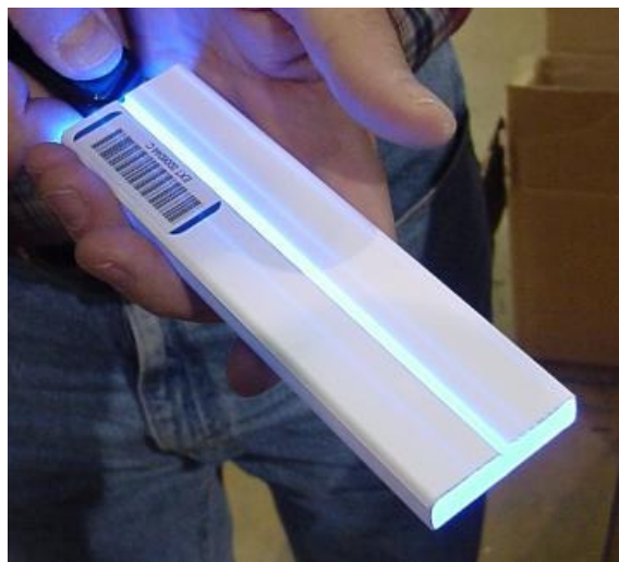
Figure 3.5: A short scintillator strip being illuminated by a blue LED [72].
