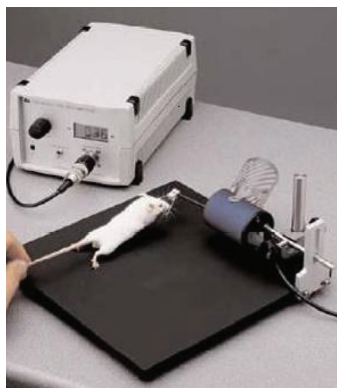
Fig. 1 - Grip strength meter for determining muscular strength in rodents.
