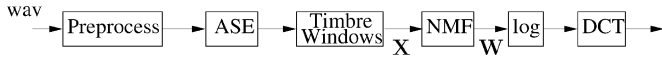
Fig. 3. Calculation of the features used for the statistical model of musical genres.
