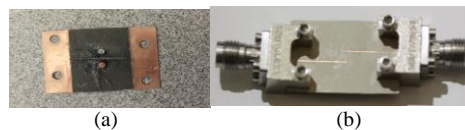
Fig. 8. (a) Photograph of 1 \times 2 Dielectric Resonator Antenna with SRR arrays, (a) top view, and (b) feedline section.
