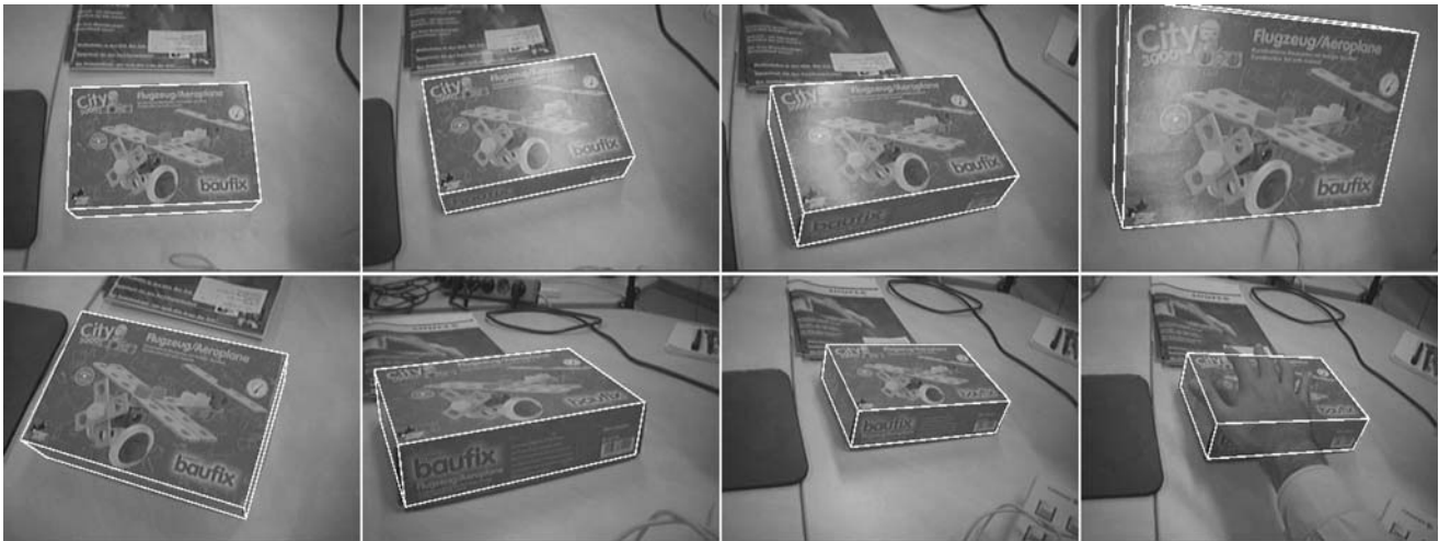
Fig. 6 Robust alignment in presence of partial occlusions, perspective and lighting effects
