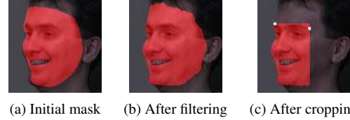
Figure 4. The mask processing for an observed image. The initial mask is essentially the texture sampling regions. It is then filtered using a joint edge-preserving filtering with the image as guidance. The final mask (c) is obtained by excluding occluded regions using 2D detected landmarks on eyebrows (the white points).
