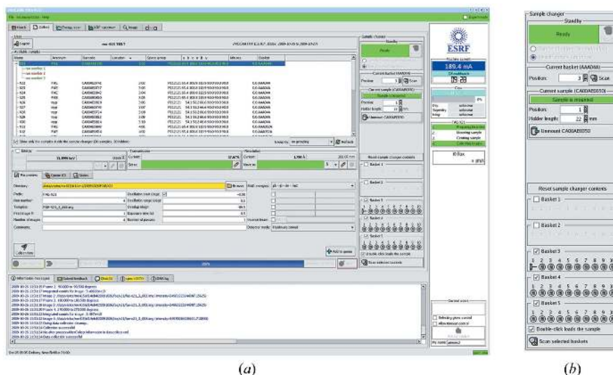
Figure 3 ( a ) The Collect tab of the MxCuBE GUI. The larger area in the top portion of the GUI shows information contained in the ISPyB LIMS (sample name, protein acronym, barcode, space group, unit-cell dimensions etc. ) for the samples contained in the SC3 sample changer. ( b ) The sample-changer brick embedded in the Collect tab. The two-dimensional barcodes of the SPINE standard pins contained in the SC3 are read by clicking 'scan selected baskets'. The sample currently mounted is flagged in both the sample changer brick and in the sample area (shown in bold green). In this figure MAD/SAD data collection (see text) is not activated.
