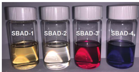
Fig. S2. Solutions of polymers in the SBAD series in chloroform (0.4 mg/mL).
