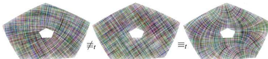
Fig. 2. Homotopy for direction fields: the middle field is homotopic to the one on the right but not to the one on the left (they can not be transformed continuously one into another)
