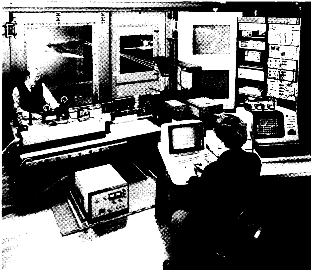
Figure 7. Laser velocimeter setup in 7- by 10-foot wind tunnel.
