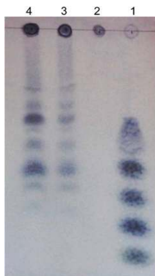
Fig. 7 Thin layer chromatography (TLC) of hydrolysis products of 0.7 % (w/v) barley- \beta -D-glucan. Lanes: 1 glucose, cellobiose, cellotriose, cellotetraose, and cellopentaose markers; 2 barley- \beta -D-glucan with inactivated (at 100 °C for 5 min) purified PgluE8; 3 barley- \beta -D-glucan hydrolyzed by purified PgluE8 for 1 h in a 1.0 U/mL reaction system at 50 °C and pH 5.5; 4 barley- \beta -D-glucan hydrolyzed by purified PgluE8 for 3 h in a 1.0 U/mL reaction system at 50 °C and pH 5.5
