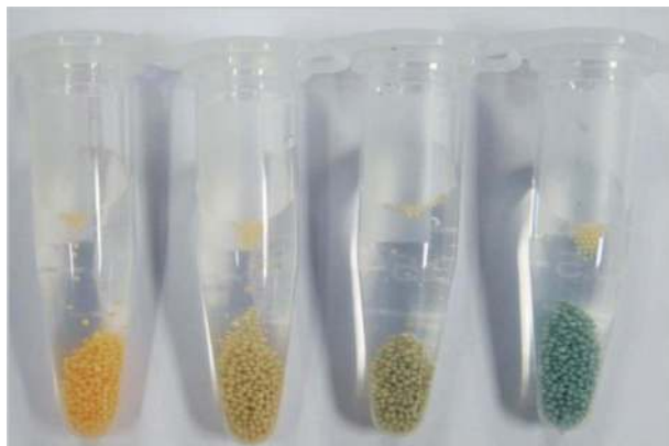
Fig. 6 The color of the BF 2 -curcumin-coated resin in the pond water sample spiked with As(III) in concentrations of 0, 3 \times 10^{-5} , 5 \times 10^{-4} and 1 \times 10^{-3} M, from left to right.
