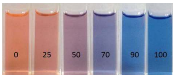
Fig. 3 The color of BF 2 -curcumin solution in various concentrations of As(III) solution between 0 and 100 μM As(III).
