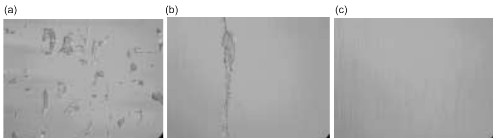
Figure 18. Nomarski microscopic images of ground surfaces at different current duty ratios. (a) Surface damage ( R_c = 20\% ); (b) surface crack ( R_c = 40\% ); (c) defect free surface ( R_c = 50\% ).
