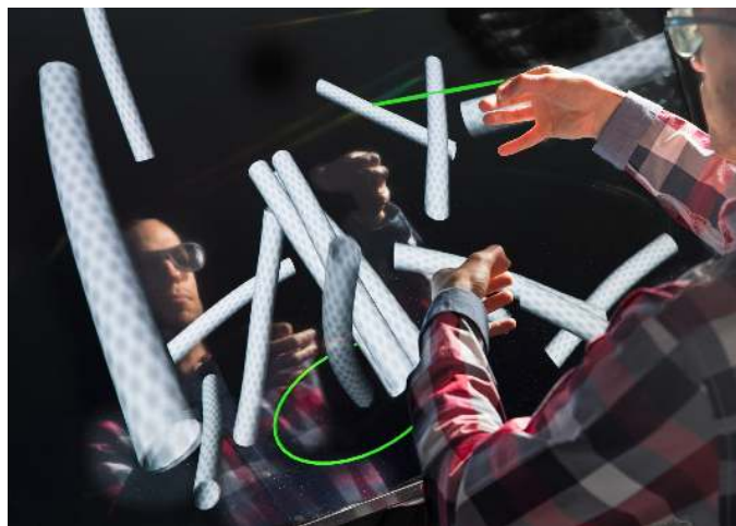
Fig. 3. A user interacts with NanoSim. Forming a ring with the index finger and thumb activates a “grab” event in the corresponding position in the virtual space, indicated by a green ring. The “grab” gesture allows the user to clasp and move the virtually attached nanotube. ©Thor Balkhed.
