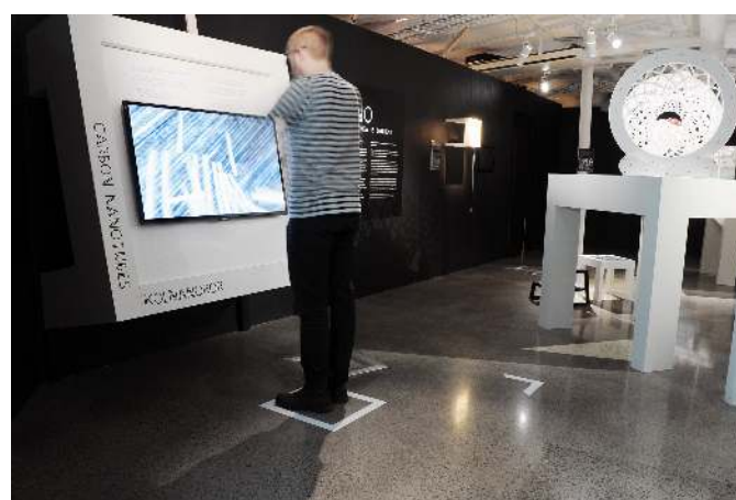
Fig. 2. A user actively interacts with the NanoSim system embedded in the NANO exhibition. The white square on the floor indicates where users should stand for optimal gesture detection and head tracking by the overhead depth camera. The corner angle indicates the boundary of the detection area. Photo: Anders Ristenstrand. ©NVAB, Sweden.
