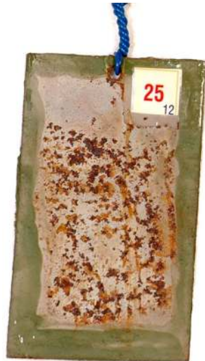
Fig. 5 Salt spray tested nickel deposited panel
