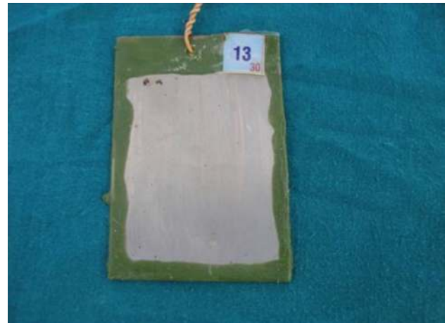
Fig. 6 Salt spray tested nickel–copper alloy deposited panel
