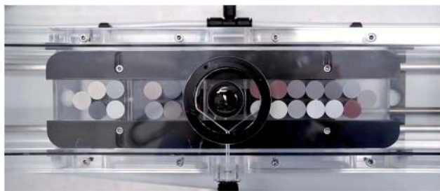
Fig. 1 Nano-particulate powder tablets (13 mm) loaded into the Zurich-type large-volume ablation cell. In the centre is a 1" mount with polished NIST SRM610-614 glass standards in epoxy.
