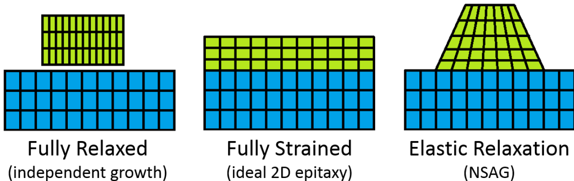
Figure 5. The concept of Nano Selective Area Growth. (left) the blue substrate lattice and green layer lattice are shown in their fully relaxed states. (right) ideal 2D heteroepitaxy, in which the epilayer strains its lattice to accommodate that of its substrate. In practice, this is impossible for large lattice mismatches and will result in threading dislocations in the epilayer as shown in Figure 3. (left) NSAG allows the lattice to elastically relax with each subsequent monolayer of growth, resulting in high quality nanostructures.
