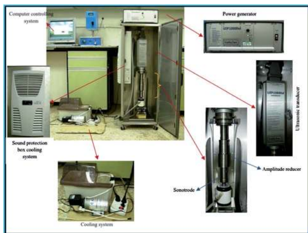
Fig. 4 nZVI synthesis using ultrasound sonication process; adapted from Jamei et al. (2012). 26
