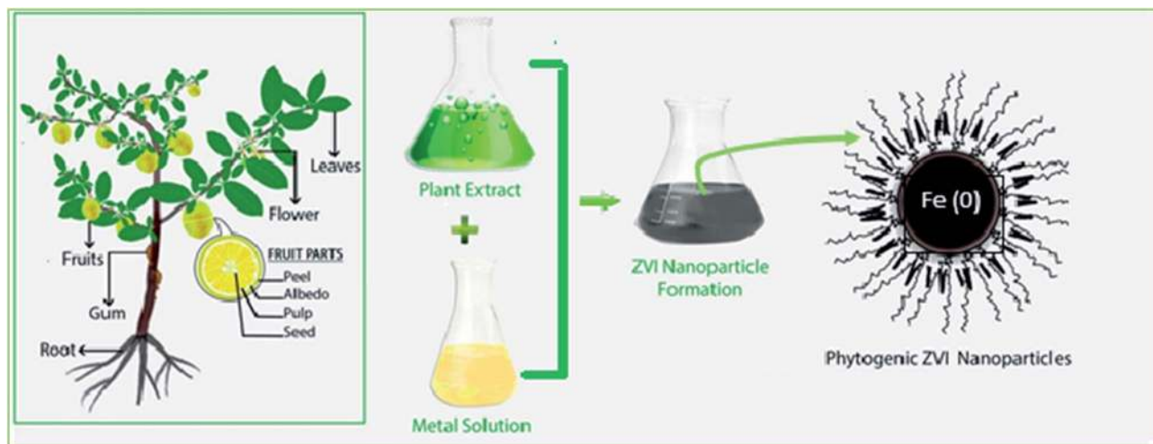
Fig. 7 Synthesis of nZVI from plant extracts; modified from Puthukkara et al. (2020). 33
