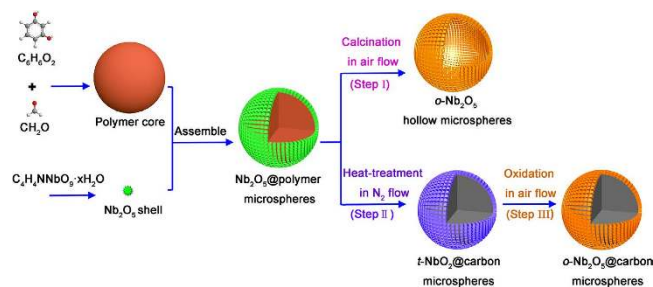
Figure 1. Schematics of the fabrication process: amorphous \text{Nb}_2\text{O}_5 @polymer core-shell microspheres were obtained through hydrothermal method, followed with different post-treatments: (Step I) calcination in air flow at 600^\circ\text{C} ; (Step II) heat-treatment in \text{N}_2 flow at 800^\circ\text{C} ; (Step III) a mild oxidation of t\text{-NbO}_2 @carbon microspheres in air flow at 300^\circ\text{C} .
