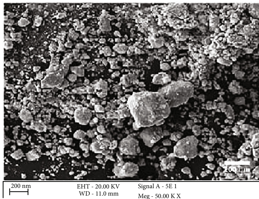
FIGURE 6: SEM image of ZnO nanoparticles.
