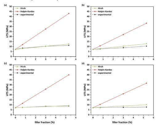
**Figure 9.** Comparison of the theoretical and experimental tensile strengths of the MMMs with (a) oxidized GNPs; (b) raw GNPs; (c) plasma-treated MWCNTs and (d) raw MWCNTs.
