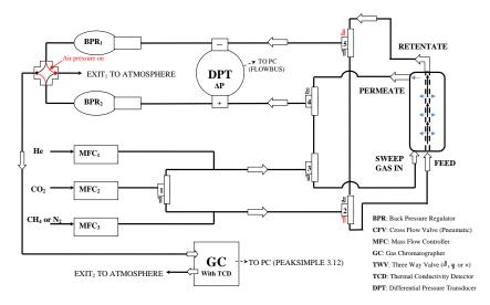
Figure 2. Scheme of laboratory apparatus for gas-separation experiments under continuous flow [32].
