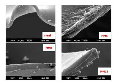
**Figure 4.** Morphology of dense neat Pebax-1657 and nanocarbon-based Pebax-1657 mixed matrix membranes.
