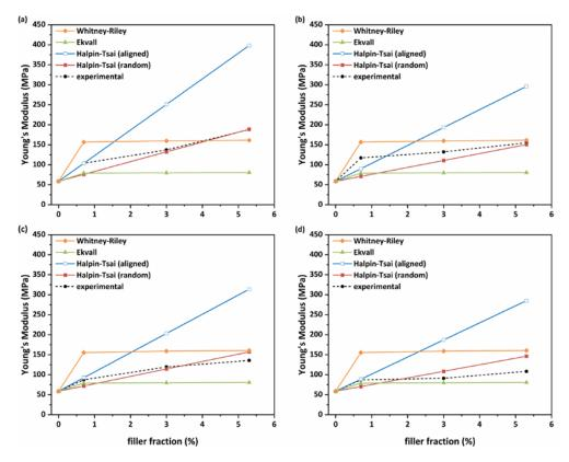
**Figure 8.** Comparison of the Young's modulus as theoretically calculated from the Halpin–Tsai, Ekvall and Whitney–Riley models and from the experimental data for MMMs with (**a**) oxidized GNPs; (**b**) raw GNPs; (**c**) plasma-treated MWCNTs and (**d**) raw MWCNTs.
