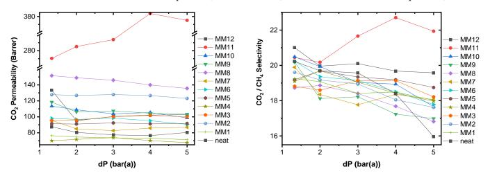
**Figure 10.**  $CO_2$  permeability (left) and  $CO_2/CH_4$  separation factor (selectivity) (right) versus pressure drop across all studied MMMs for 10% v/v CO<sub>2</sub> in CH<sub>4</sub>. Temperature was kept constant at 298 K.
