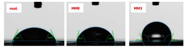
**Figure 6.** Characteristic images of water contact angles on three membrane surfaces.
