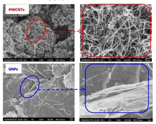
**Figure 3.** SEM images of raw multi-walled carbon nanotubes (MWCNTs) and graphene nanoplatelets (GNPs).
