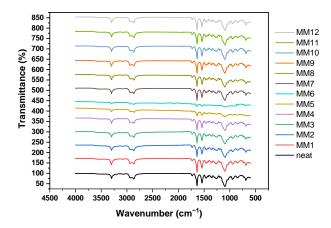
**Figure 5.** FTIR spectra of the thirteen Pebax-1657 membranes, the neat and the twelve mixed matrix membranes.
