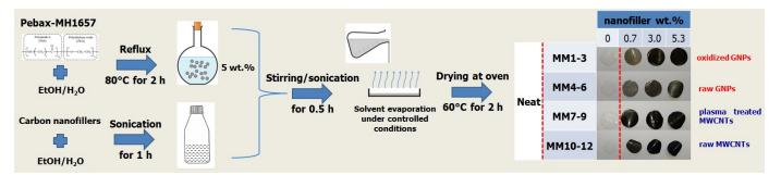
Figure 1. Schematic representation of all intermediate steps for Pebax-1657-based MMM production.
