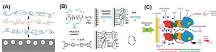
Fig. 3. Schematic illustrates the formation of LbL coatings using different methods. (A) Electrostatic interactions; (B) hydrogen bonding; or (C) biological interactions. Figures adapted from ref. 13 and 71 .
