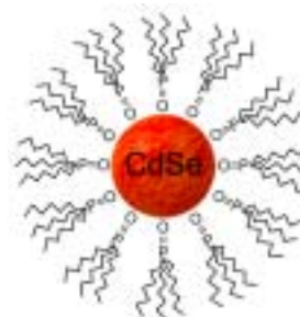
Figure 1. An organometallic reaction used to fabricate CdSe NQDs surface passivated with an organic capping layer; TOPO molecules of cap are shown.
