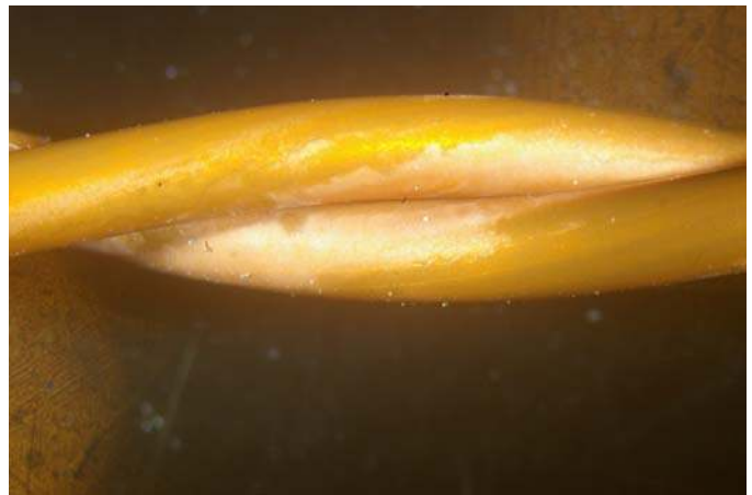
Figure 3. Damaged area: Nanocomposite Enamel, 65% RH, 9000 V
