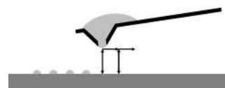
FIG. 1. Sketch of the nanoscale dispensing (NADIS) principle. A hollow AFM tip with an aperture at its apex is loaded with liquid. By bringing the tip briefly into contact with the sample, some liquid is transferred by capillarity onto the surface (no external pressure is applied to the liquid). A SPM drives the probe, so that high accuracy is provided in the positioning of the droplets.
