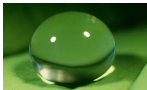
Fig. 1. A droplet on a superhydrophobic surface: The droplet touches the leaf only at a few points and forms a ball. It completely rolls off at the slightest declination. Adapted from reference [16] with permission.
