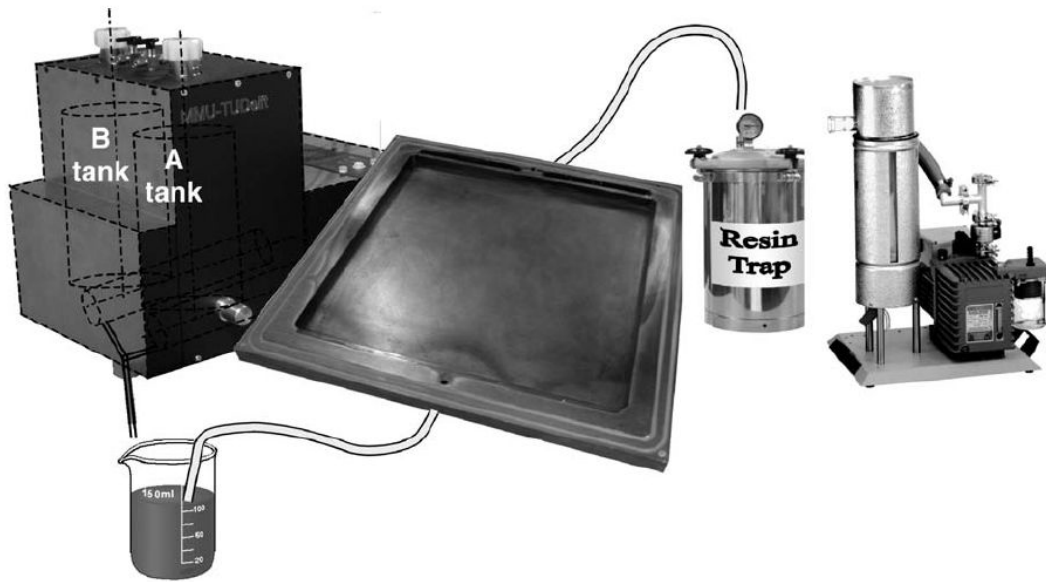
Figure 3 Infusion equipment - from left to right: Mini Mixing Unit “MMU-TU Delft”, resin reservoir, stainless steel infusion mould, resin trap, cold trap and vacuum pump [24].
