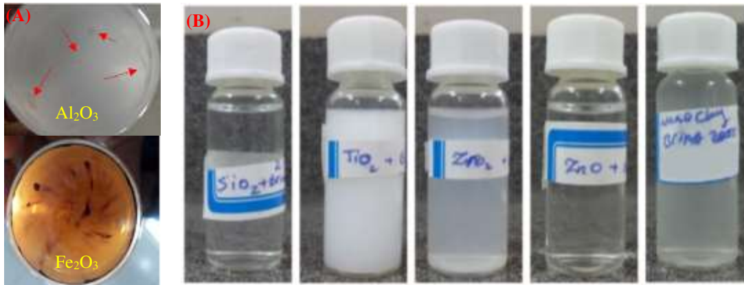
Figure 7. (A) Significant precipitation of Al_2O_3 and Fe_2O_3 nanofluid after 30 min, (B) SiO_2 , TiO_2 , ZrO_2 , ZnO_2 and nanoclay nanofluid after one hour (base fluid: 20,000 ppm diluted formation water, FW2, NP: 0.05 wt%, guar gum polymer: 0.05 wt%)
