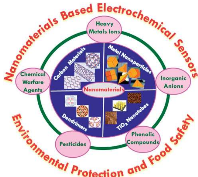
Fig. 3 Schematic of the electrochemical detection of chemical contaminants with nanomaterials.
