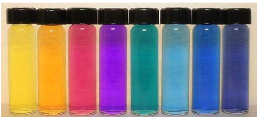
Figure 1.5 Digital image of colloidal silver nanoplates with different colors. Adapted with permission from Ref. 72. Copyright © 2012 WILEY-VCH Verlag GmbH & Co. KGaA, Weinheim
