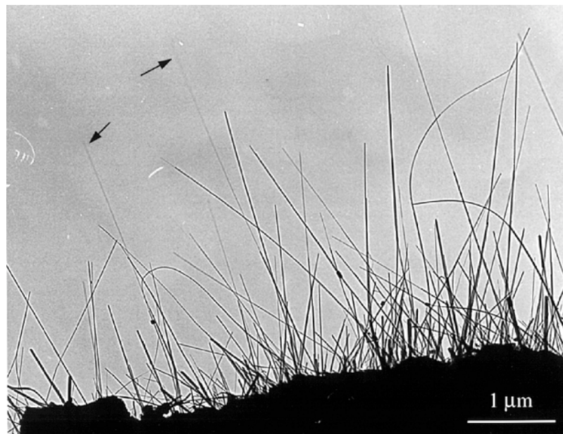
Fig. 3 A typical TEM image showing the multi-walled carbon nanotubes produced by arc-discharge, that were used for the measurements presented in this paper.
