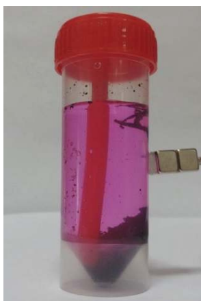
Fig. 2. Investigation of the magnetic susceptibility of the granules distributed in the liquid
