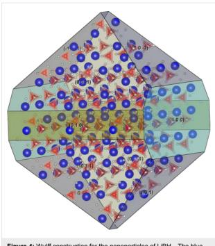
Figure 4: Wulff construction for the nanoparticles of LiBH<sub>4</sub>. The blue spheres are for lithium, red for boron and white are hydrogen atoms.
