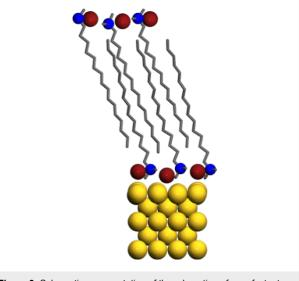
Figure 3: Schematic representation of the adsorption of a surfactant on a gold surface. Spheres represent gold (yellow), silver (grey) and bromine (red) and the tails of the surfactant are represented by sticks.
