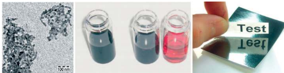
Figure 6. TEM images of 1a nanoparticles (left). Macroscopic appearance of the polyacetylene dispersion (center) (polymer solids content 6.4 wt %; left to right, undiluted, 10 3 - and 10 4 -fold dilution). Film prepared by spreading and drying the dispersion on white paper (right). Reprinted with permission from ref 166. Copyright 2006 John Wiley & Sons.
