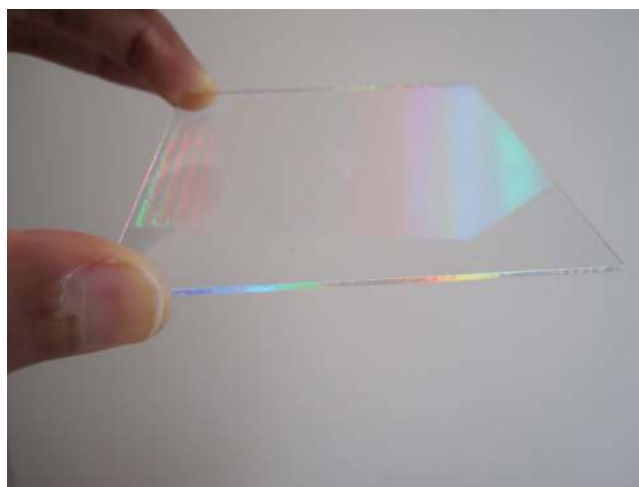
FIG. 2. A glass slide with an imprinted light trapping pattern on the surface. The pattern traps light effectively inside the glass, making it bounce back into the glass everytime it hits the glass-air interface. As a result, light is trapped and is directed to the edges of the glass slide, as can be seen here.
