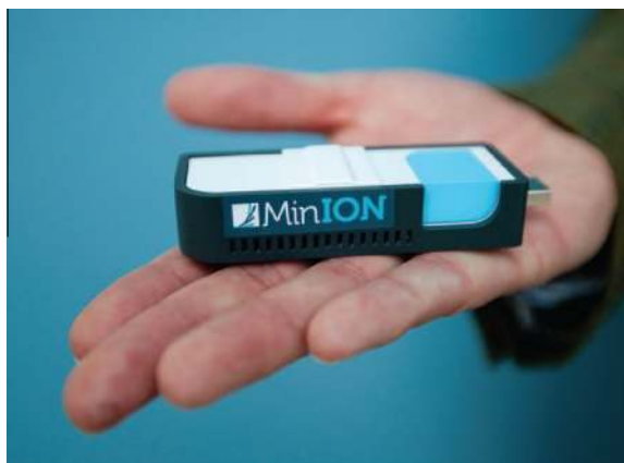
Figure 3 The portable MinION — the first handheld nanopore DNA sequencer
