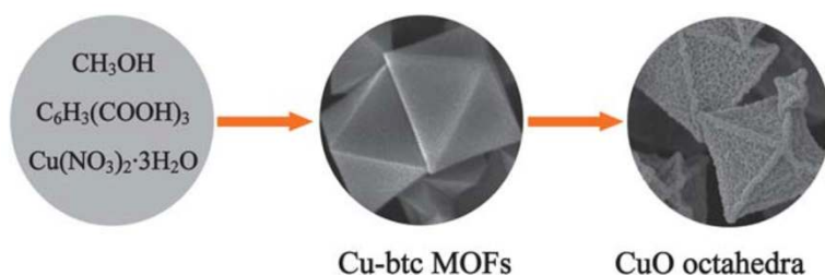
Fig. 10. Left to right: reactants for hydrothermal synthesis to generate Cu-BTC single crystals, which can then be converted into porous CuO octahedra via pyrolysis at 300 °C. Reprinted with permission from ref. 44 .
