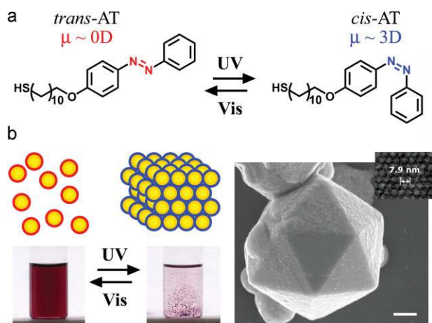
Figure 11. Self-assembly mediated by light-induced molecular dipole forces. a) Azobenzene thiol (AT) isomerizes from the trans - to the cis -conformation upon exposure to UV light. Importantly, the cis -isomer is characterized by a strong molecular dipole. [63,219] b) AT-functionalized nanoparticles self-assemble into various ordered structures in the presence of UV light due to molecular dipole interactions between the azobenzene groups tethered to their surfaces. Exposure to intense visible light induces the re-isomerization of the AT groups to the trans -conformation, and the loss of dipole–dipole interactions results in the dissolution of the NP structures. [63,219]
