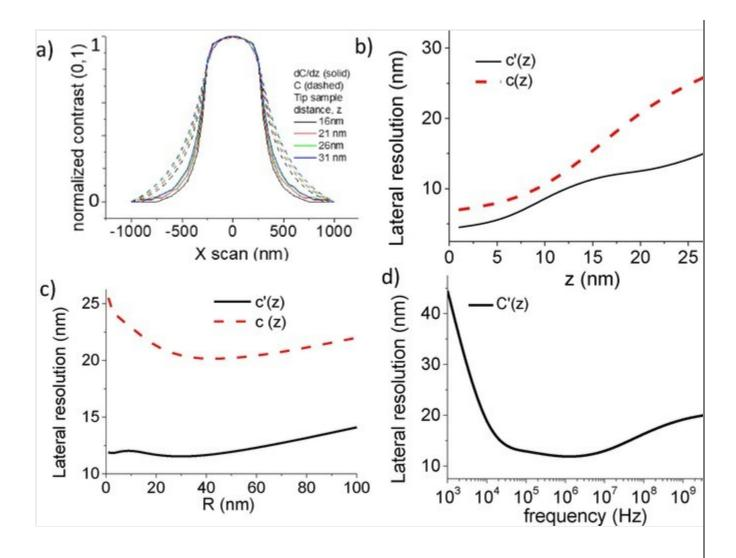
Experimental comparison of EFM lateral resolution and electrical contrast at different frequencies.
